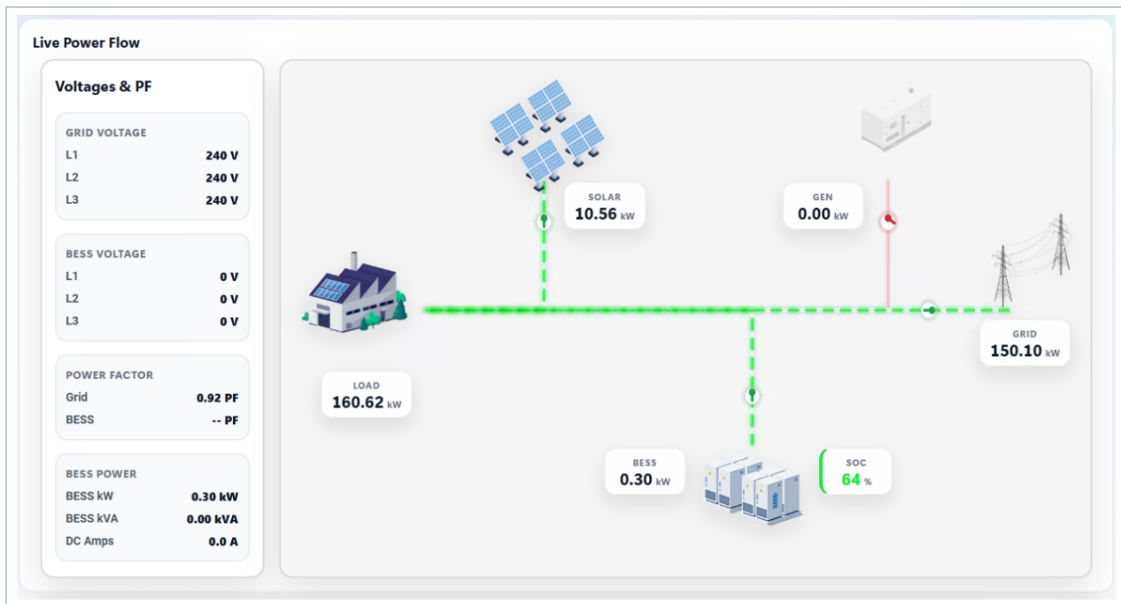
Figure 7 Live Power Flow on a running site. The grid is importing 150.10 kW, solar is producing 10.56 kW and the site load is 160.62 kW; the battery is almost idle at 64 % SOC. The generator branch is drawn open (red) because the set is not running.
